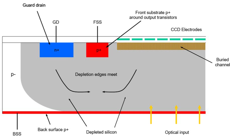
With correct bias conditions the depletion regions from the CCD channel and the guard diode merge to block the conductive path, rather like the operation of a JFET, as shown above. If incorrect, then there is a direct resistive path between the front and back contacts and excessive currents can flow, as shown below.
