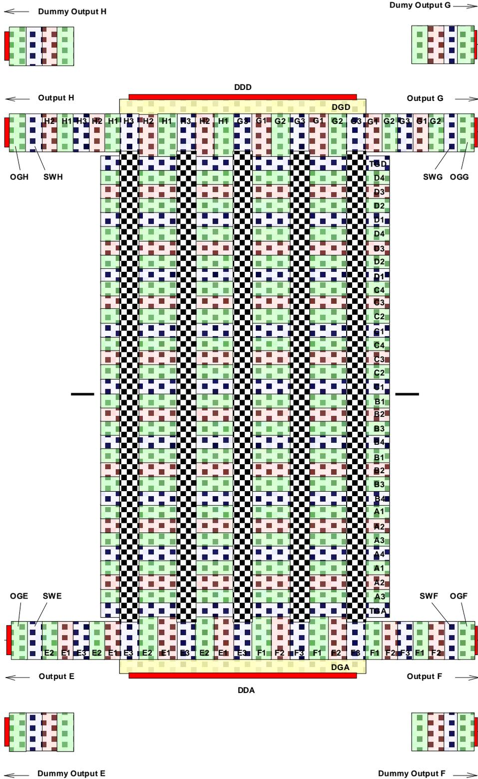
The IMC implant is under image phases A4, B4, C1, D1 and the transfer gates as shown below.
