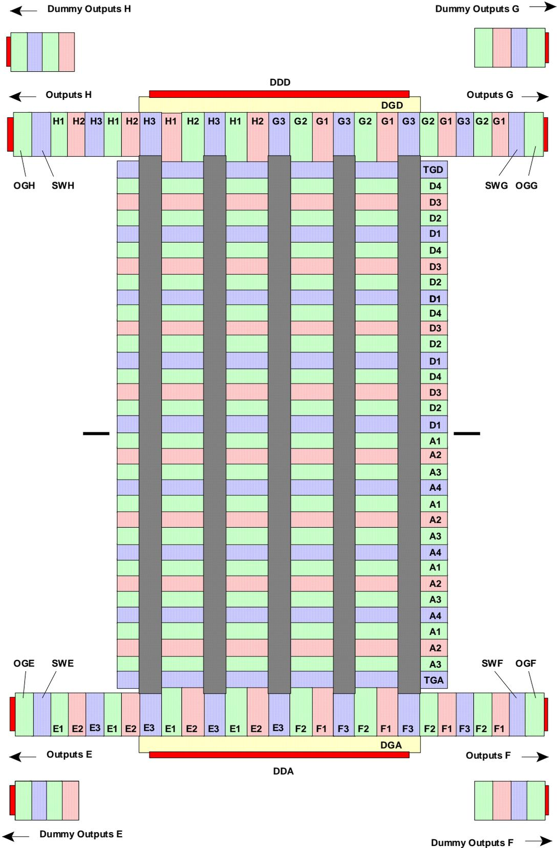
The IMO implant is under image phases A4, B4, C1, D1 and the transfer gates as shown below.
