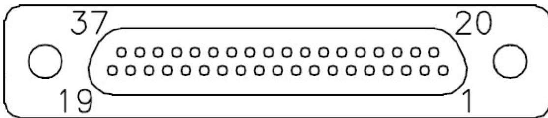
This numbering applies to all connectors. The connector is a Glenair 37P micro D type.
