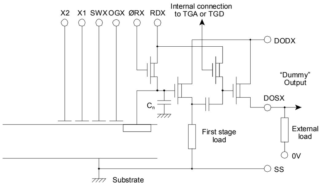
The first stage load of each output (real or dummy) draws a quiescent current of approximately 0.2 mA via SS.
