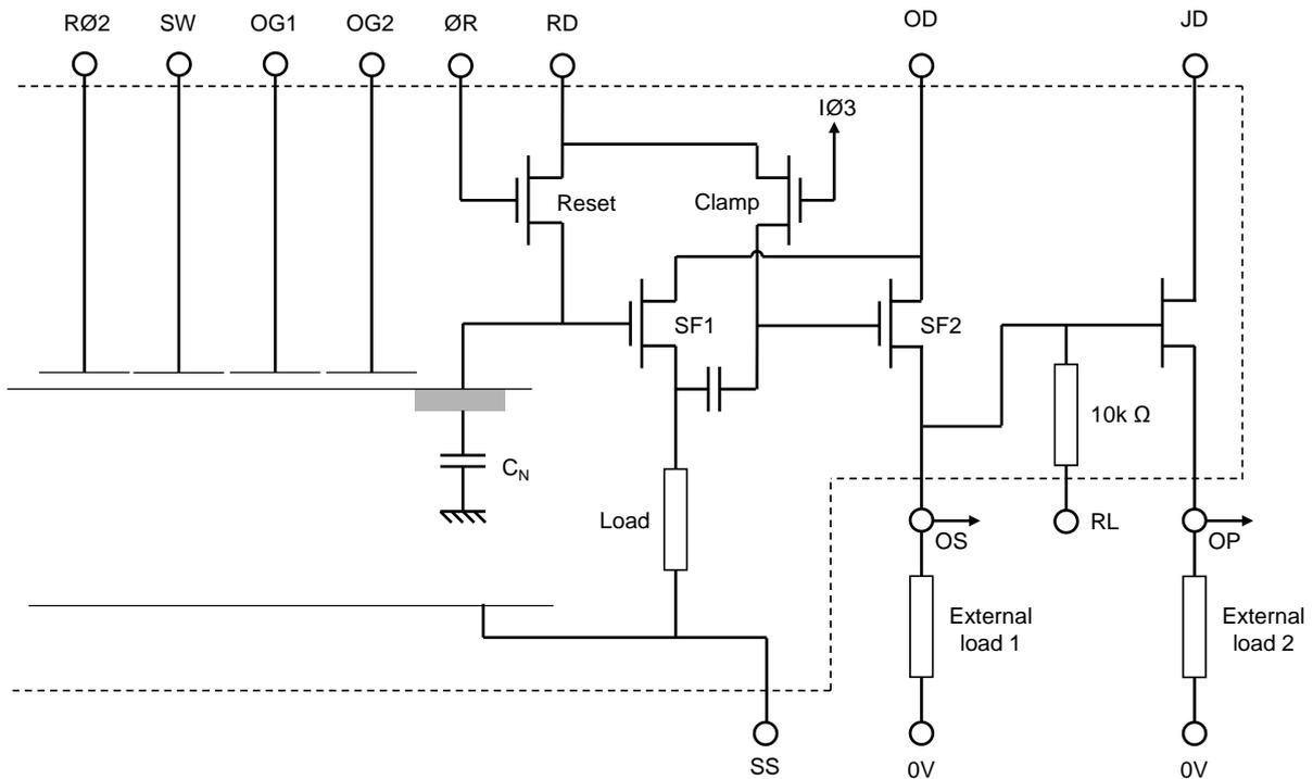
The device has a conventional output circuit with the output at OS. Within the package is an additional U309 JFET buffer amplifier for optional use, e.g. in cases where the external load capacitance is large ( $\gg 20$  pF). The connections for the left and right amplifiers are designated by the suffix (L) and (R), respectively, not shown above.
